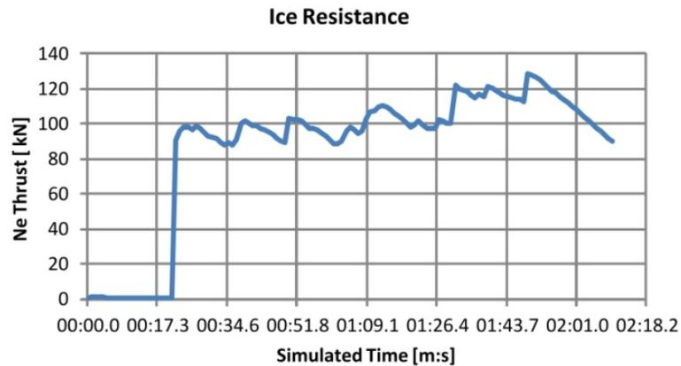
Figure 6.20: Net thrust during simulation in 35% coverage. [11]
