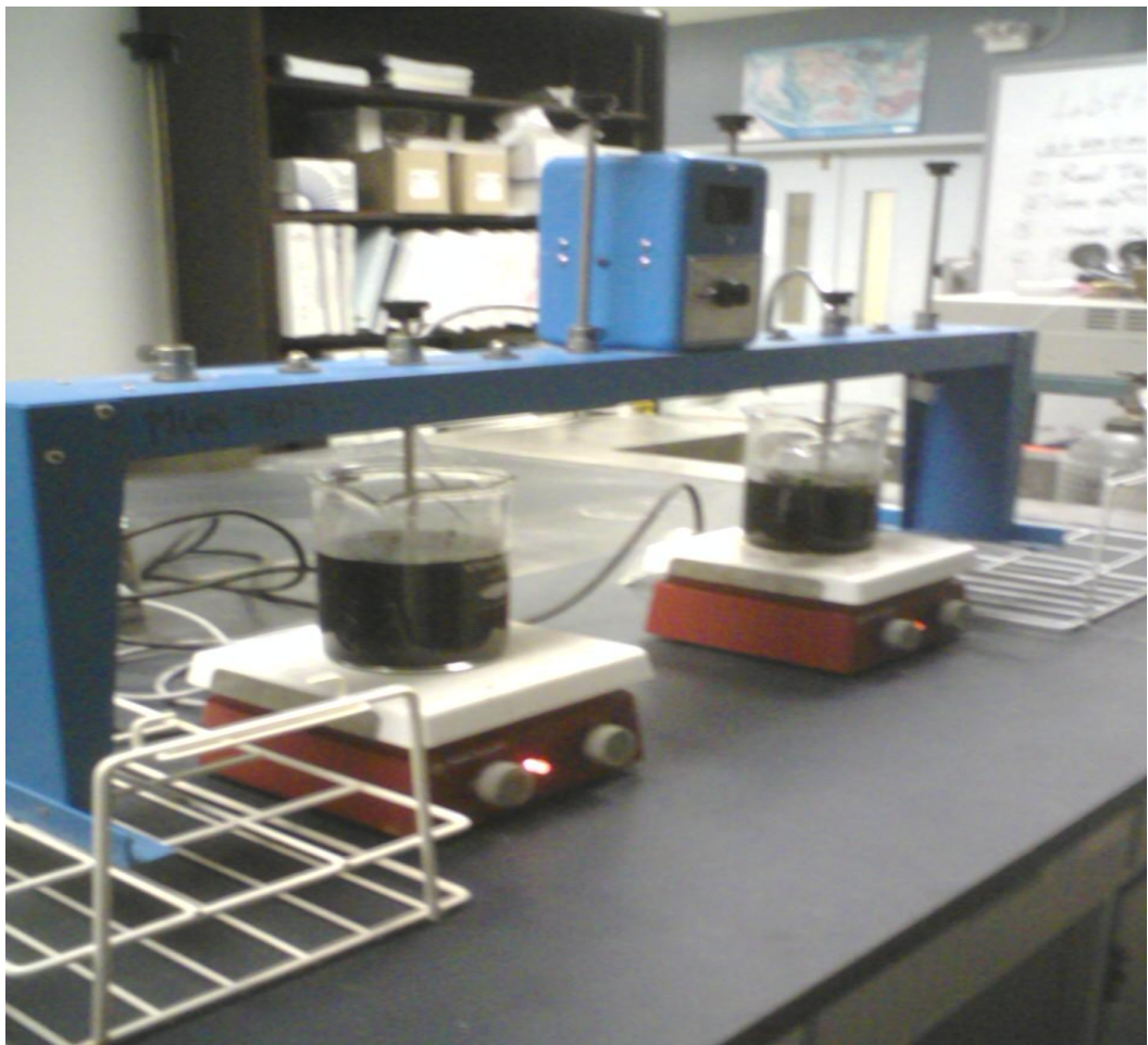
Figure C-3 Sample laboratory setup used to clean HOFA
