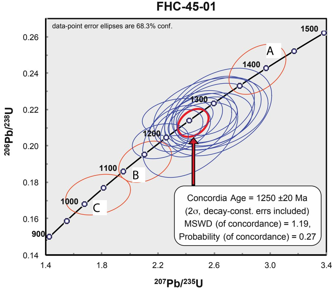
Figure 2-19: LA-ICPMS U-Pb zircon data for sample FHC-45-01 plotted on a Concordia diagram. Fifteen analyses shown in blue ellipses give a Concordia age of  $1250 \pm 20$  Ma ( $2\sigma$ ). Three analysis labeled “A”, “B” and “C”, shown as orange ellipses, are excluded from the age calculation.
