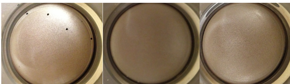
Figure 2-12 Corrosion results after 20 days immersion
