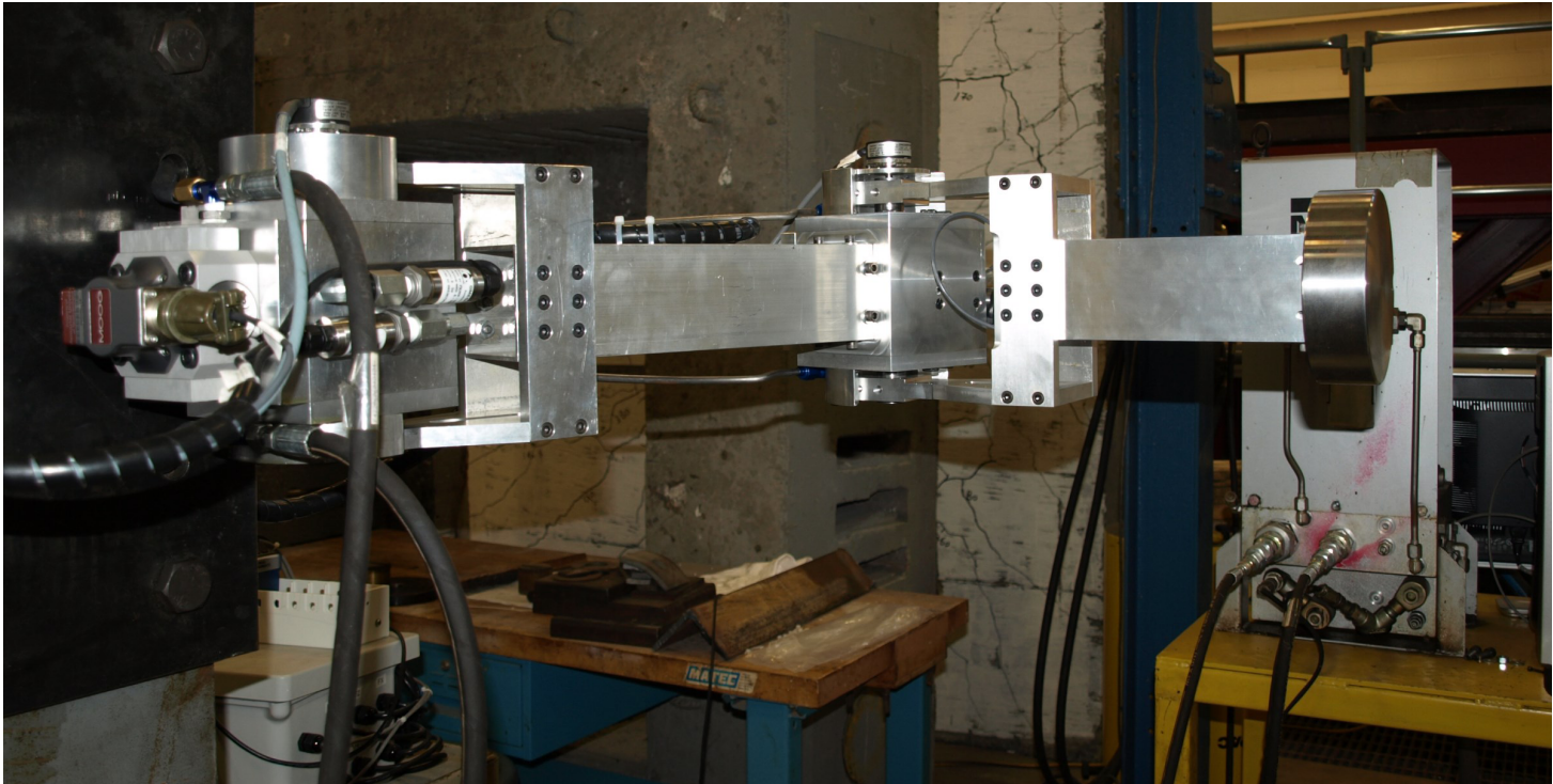
Figure 3.19: The proposed robotic manipulator after fabrication
