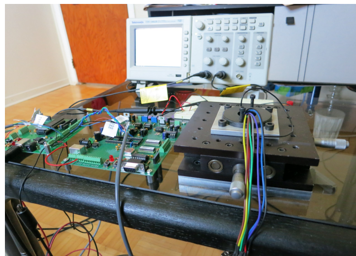
Figure 5.12: Selected photos from the calibration of the 2-D PSD
