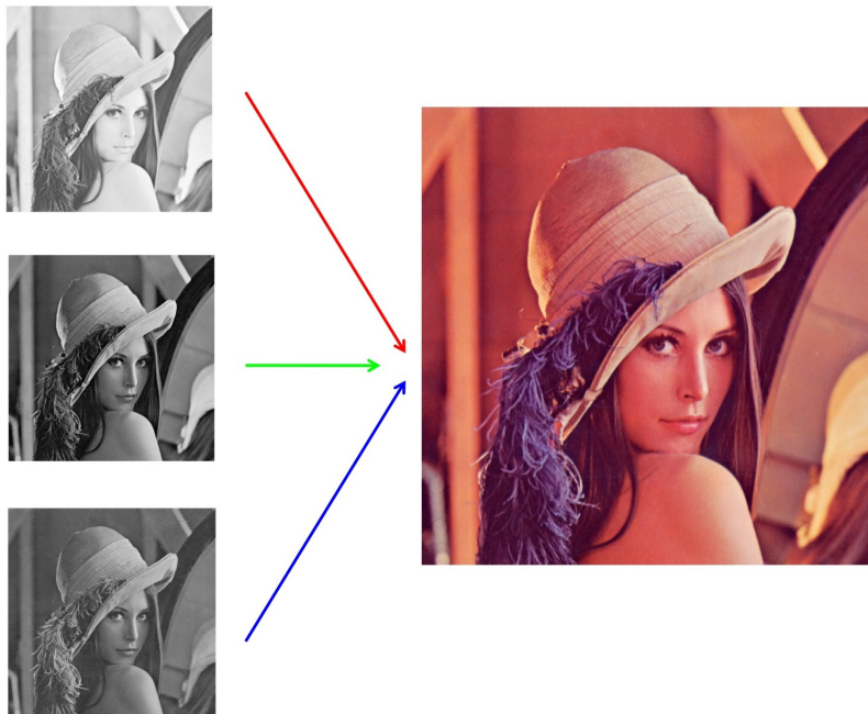
Figure 4.5: Combining 3 Channels to form a Color Image
