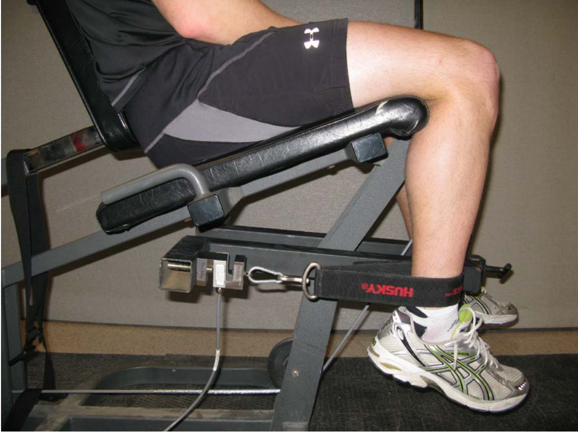
Figure 2. Photo of Leg Extension Custom Apparatus
