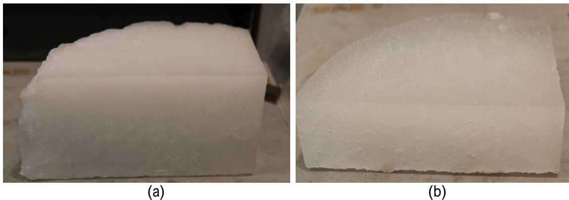
Figure 3.17: (a) Vertical and (b) Horizontal cut of crushed ice sample
