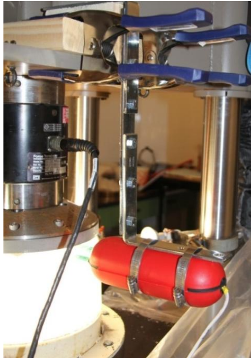
Figure 3.14: Arrangement of Tekscan sensor with MTS load frame
