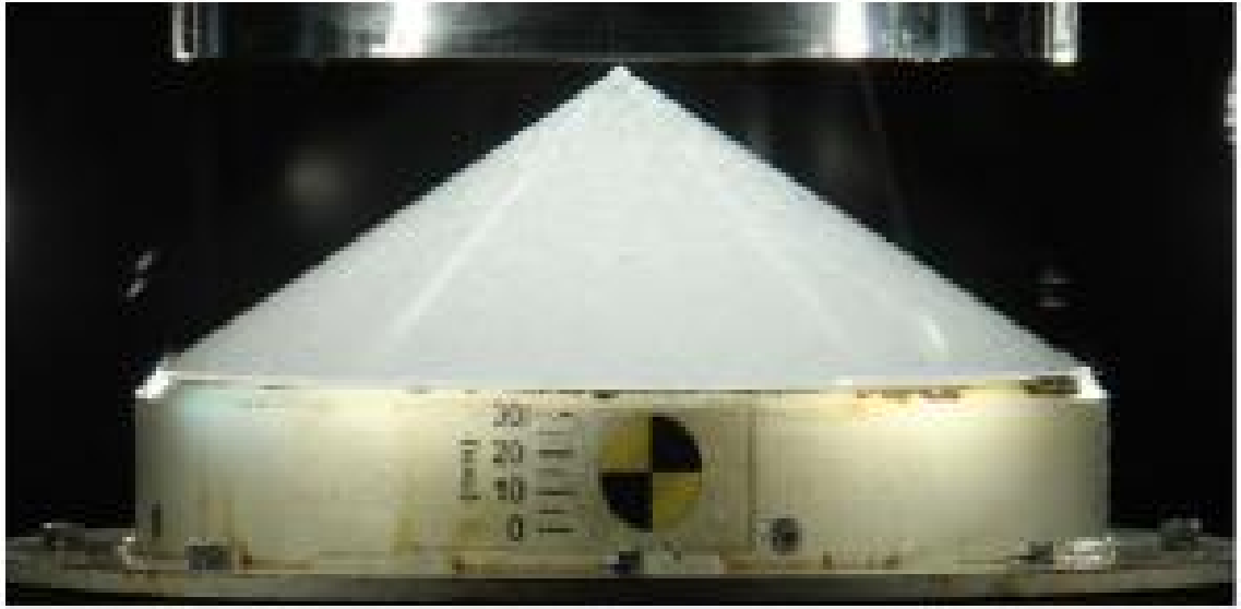
Figure 3.12: Ice sample of 30° cone angle (Dillenburg, 2012)
