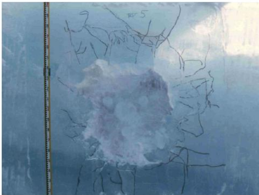
Figure 2.12: Brittle failure observed for fast test ( v=1.0 cm/s) during Rae Point experiments with 1\text{ m}^2 spherical indenter (Masterson et al., 1999)
