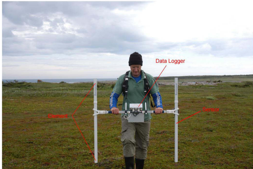
Figure 3.3: The fluxgate gradiometer used at Phillip's Garden with components labelled. Photo: PAC Archaeology Project.
