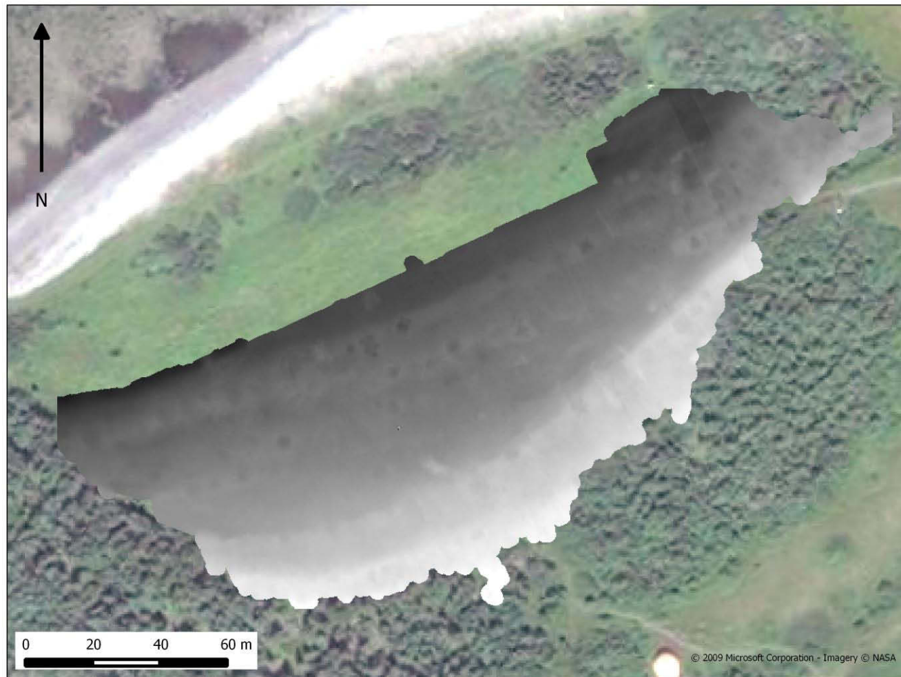
Figure 3.7: The IDW raster produced for the survey at Phillip's Garden. The darker areas are the lower elevations, with lighter areas representing the higher ground. Note the darker circles which are the depressions. The white circle (bottom right) is the Park's Canada yurt.
