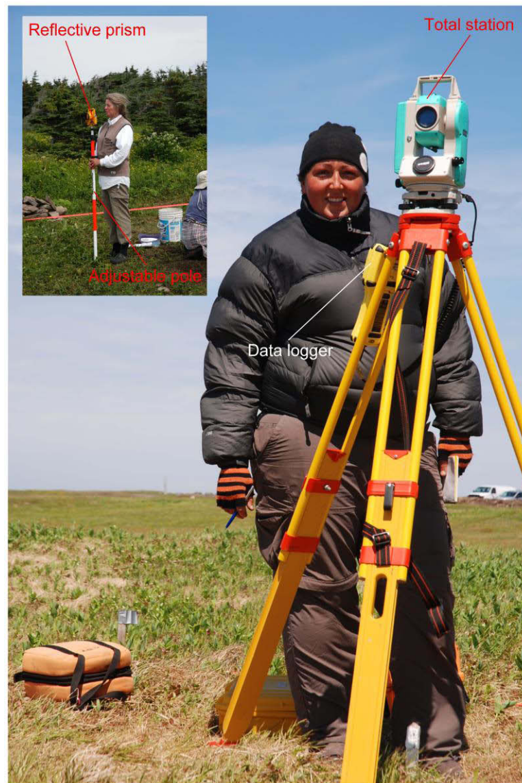
Figure 3.2: The Nikon NIVO 3.0 used at Phillip's Garden with components labelled. Photo: PAC Archaeology Project
