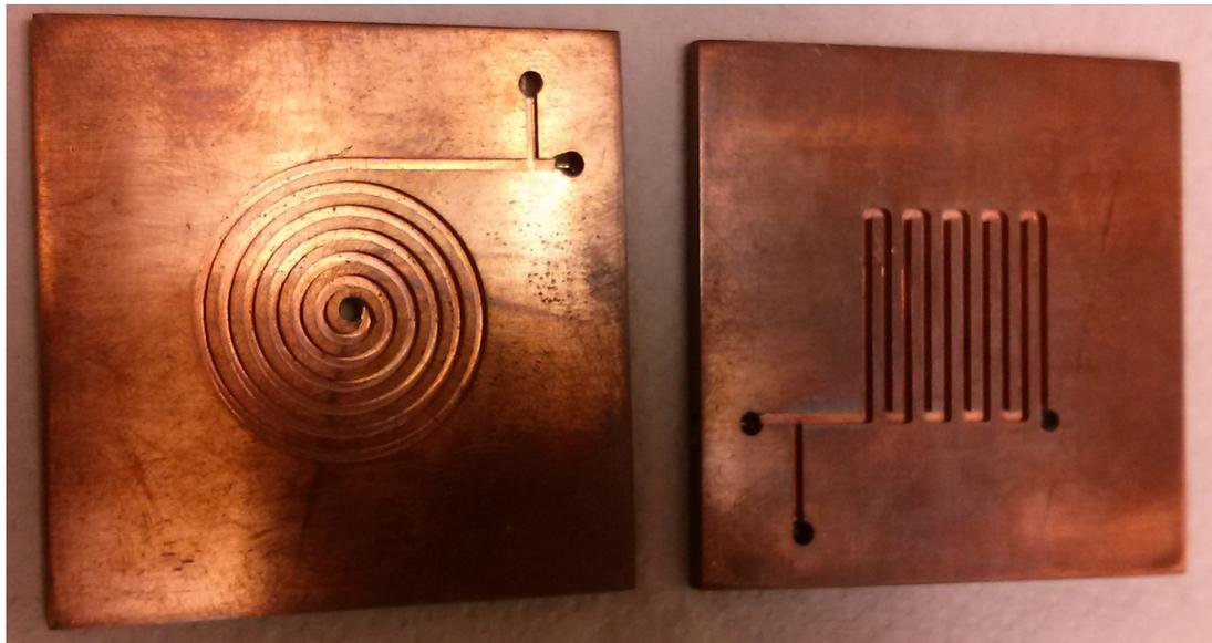
Figure A.1: Heat sinks channel patterns
