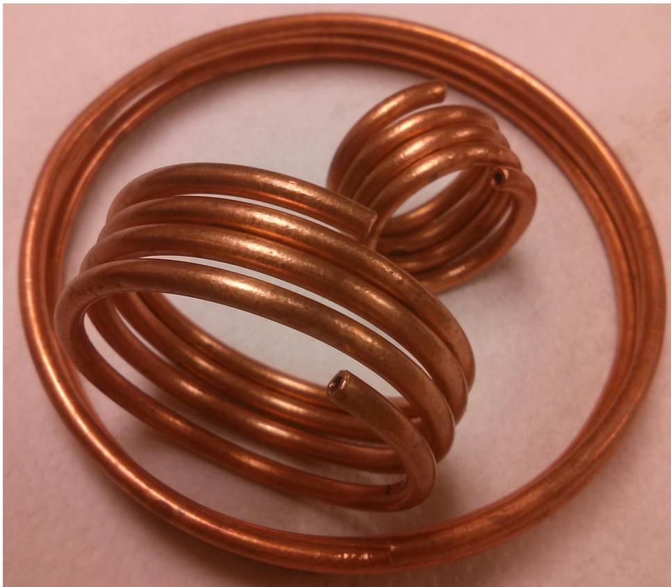
Figure A.4: Coiled tubes used for the heat transfer experiments in Chapter 7
