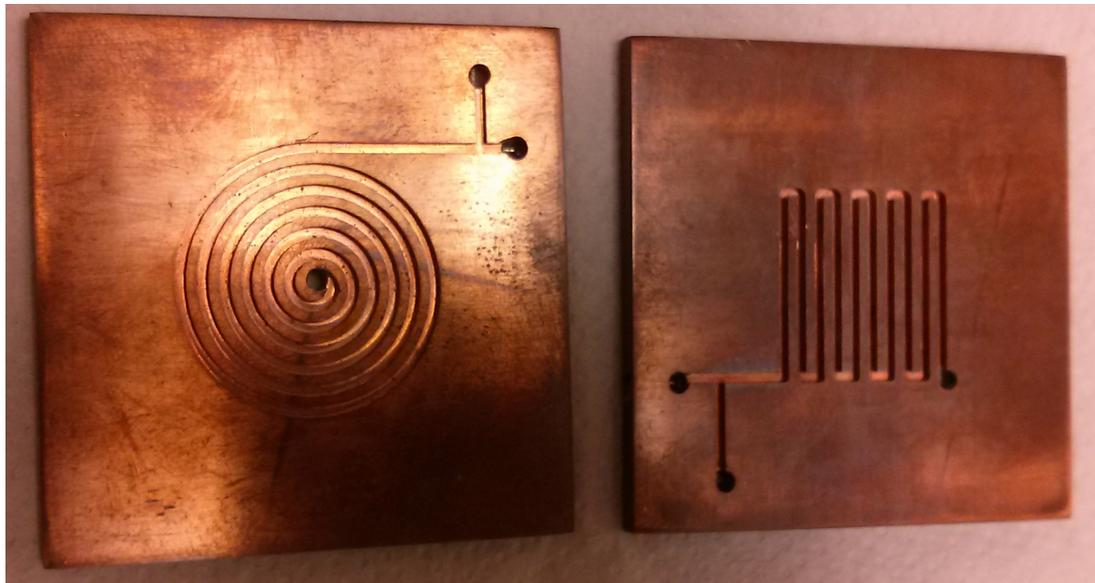
Figure 4.1: Spiral and straight heat sinks used in the experiments
