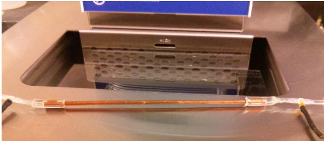
Figure A.6: The straight tube used for the heat transfer benchmarking test
