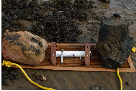
Figure 3.13: The pressure sensors were RBR Tide and Wave Recorders. They were moored to the flats on small grates.
