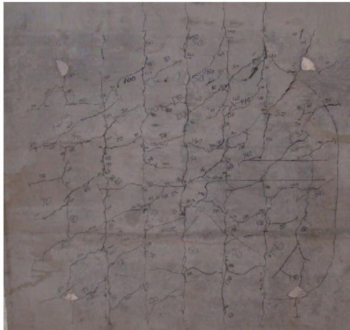
Figure 4.42. Crack patterns of the test slab HFR250-0.96/0.2
