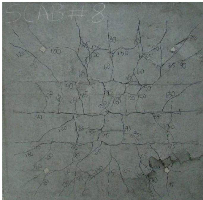
Figure 4.36. Crack patterns of the test slab HFR200-0.68/0.2
