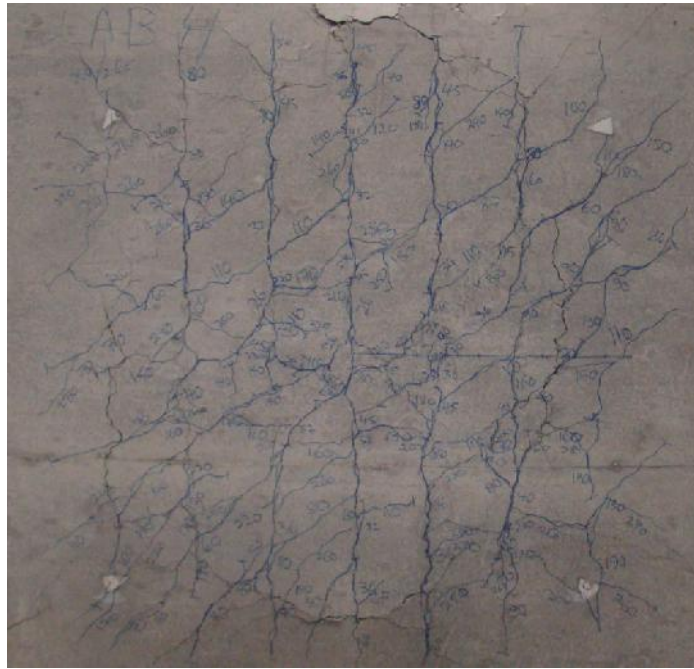
Figure 4.41. Crack patterns of the test slab HFR250-0.8/0.2
