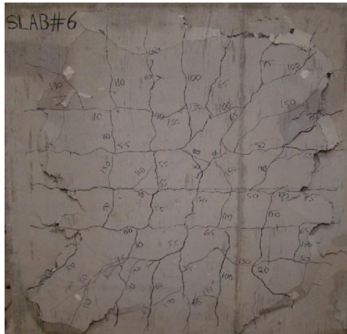
Figure 4.39. Crack patterns of the test slab R250
