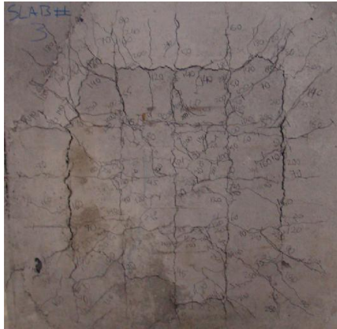
Figure 4.37. Crack patterns of the test slab HFR200-0.8/0.2
