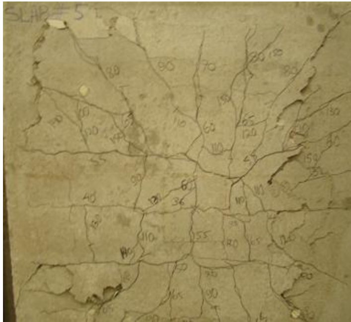
Figure 4.35. Crack patterns of the test slab R200
