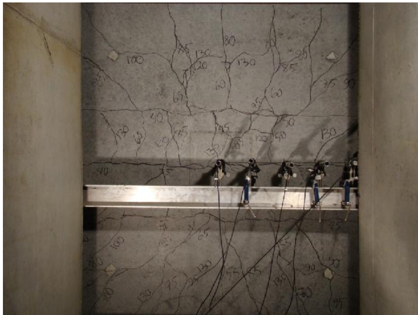
Figure 3.12. Marking the cracks on a typical slab
