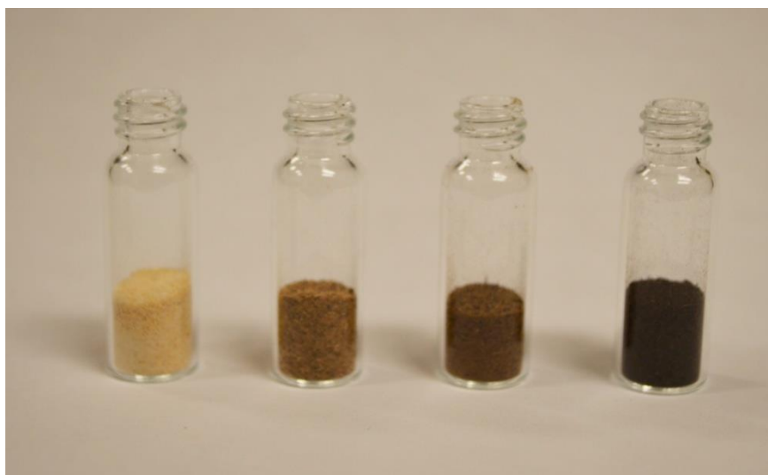
Figure 3.4: Effect of torrefaction temperature on colour of product.
