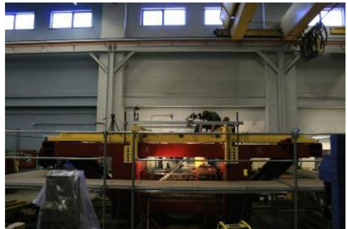
Figure 1. Full-scale steel grillage experimental setup.
