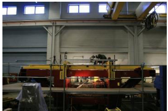
Figure 1. Full-scale steel grillage experimental setup.
