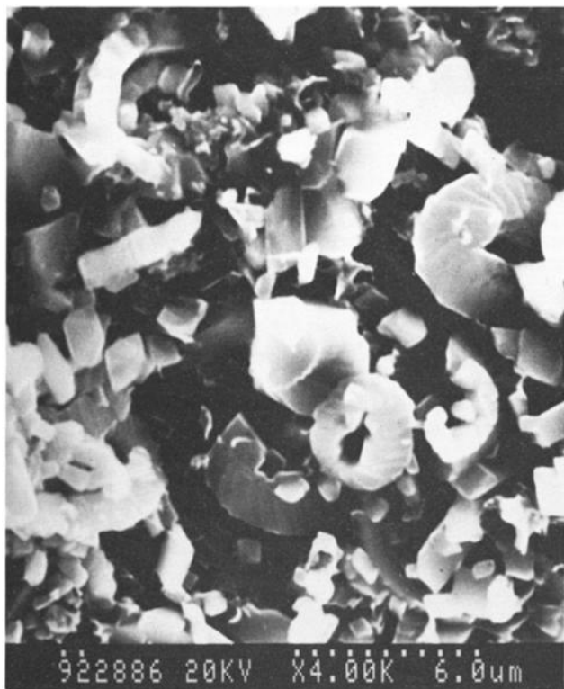
Fig. 2. Deep-sea limestone specimen 315A-21-2-11 viewed with a scanning electron microscope on a surface broken perpendicular to bedding. The dotted line indicating 6 \mu\text{m} is parallel to bedding.
