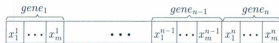
Figure 3.2: A chromosome in a GA contains n genes, where n is the number of parameters to be optimized. Each gene contains several nucleotides, which encode specific value of a parameter.
