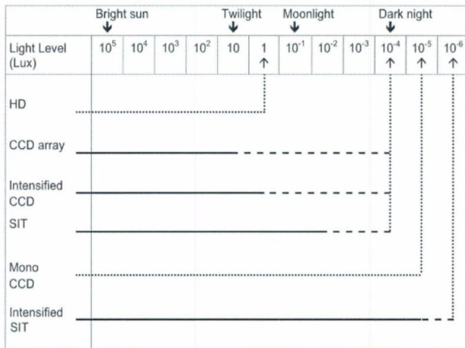
Figure 2.6 Minimum illumination levels for various camera types. Updated from Graham et al. (2004) to include high definition cameras. The solid lines are the camera minimum illumination in 1993; dashed lines indicate minimum illumination in 2004 and the dotted lines indicate the current minimum illumination.
