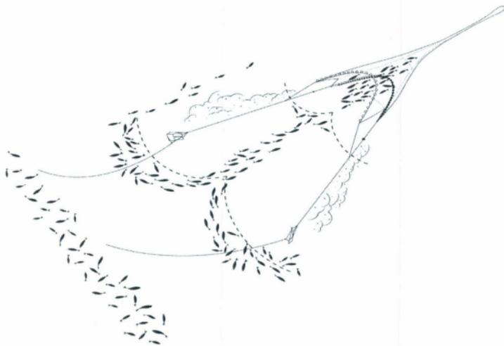
Figure 1.3 The 'fountain manoeuvre' of roundfish. The fish in front of the trawl have the potential of being herded and caught. Individuals in the sweep path will either turn around the doors into the trawl path or turn out and escape. Individuals that turned into the trawl path are herded into the mouth of the trawl. The dotted line indicates the point at which fish visually react, firstly to the doors and secondly to the mouth of the trawl (Winger et al., 2010a).
