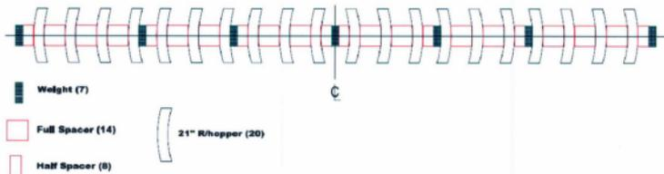
Figure 3.2 Schematic trawl plan and bosom footgear for the Goldentop trawl used by OCI vessel F/V Aqviq (Winger et al., 2010b).
