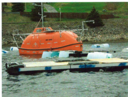
Figure 3-9: Larger artificial ice pieces built of docks and platforms
