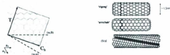
**Figure 1-14.** Schematic diagram of a SWNT with rolling vector (left) and three different types of carbon nanotubes based on the angle of chiral vector (right).<sup>32</sup>
