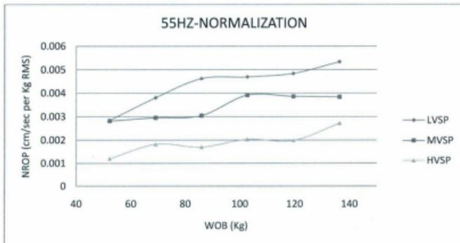
Figure 69. NROP v. WOB at 55HZ Frequency using F-RMS
