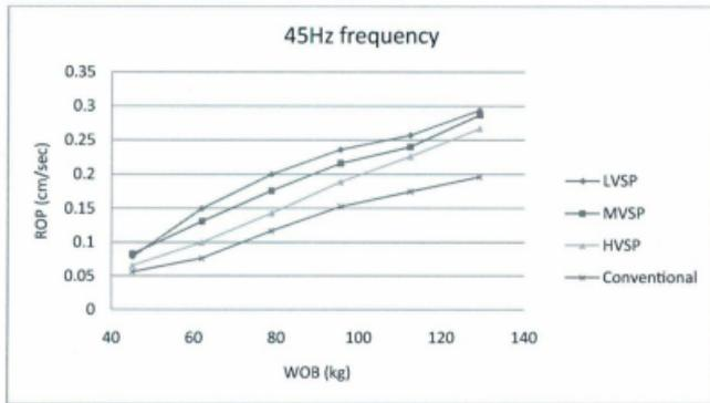
Figure 14. ROP-WOB curves at 45Hz Frequency drilling
