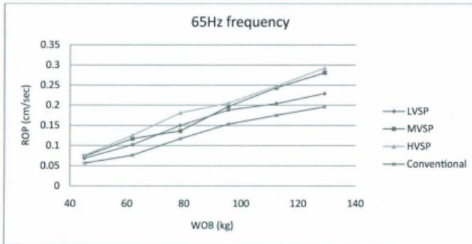
Figure 16. ROP-WOB curves at 65Hz Frequency drilling
