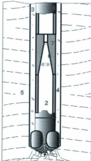
Figure 5. Schematic of vibratory rotary drilling using high frequency cavitation hydrovibrator. [1. Rock cutting tool. 2. Drilling mud. 3. Borehole. 4. Cuttings. 5. Rock. 6. Hydrovibrator shaped inner passage. 7. Hydrovibrator. 8. drilling assembly. 9. Cavity. 10. Detached part of cavity. [3].
