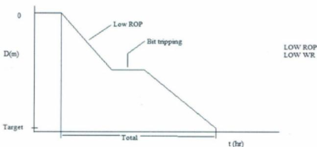
Figure 2. Low ROP, Low Wear Rate Scenario
