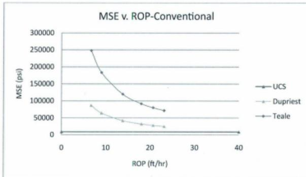
Figure 26. MSE v. ROP for conventional drilling
