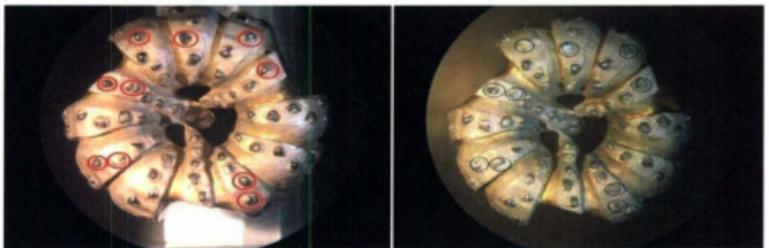
Figure 23. Plan view of diamond drag bit before (1st) and after (2nd) experiment
