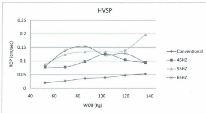
Figure 46. PDC Bit Drilling at HVSP
