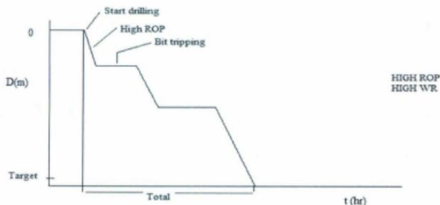
Figure 1. High ROP, High Wear Rate Scenario
