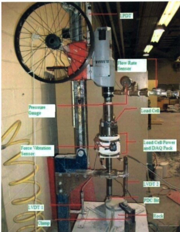
Figure 39. Modified Drilling Setup
