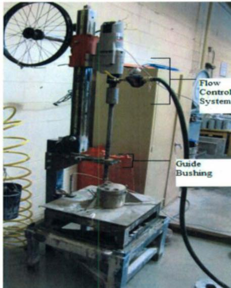
Figure 12. Drilling setup and modified drill string design
