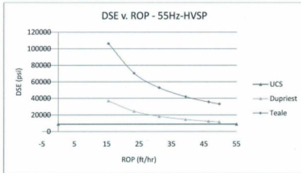
Figure 31. DSE v. ROP for 55HZ - HVSP drilling
