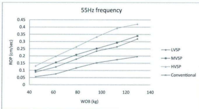
Figure 15. ROP-WOB curves at 55HZ Frequency drilling
