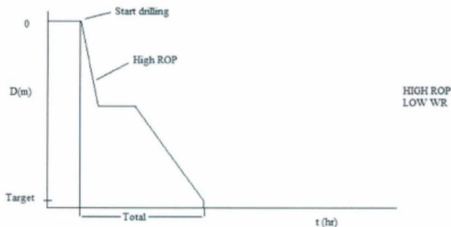
Figure 3. High ROP, Low Wear Rate Scenario
