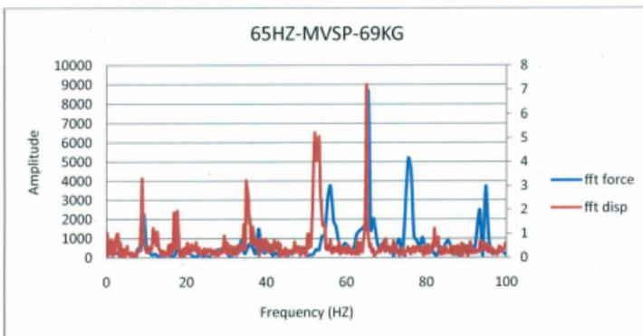
Figure 81. Force and Displacement FFT at 65Hz-MVSP-69Kg
