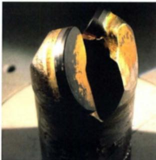
Figure 38. The 1.00-in diameter PDC Bit
