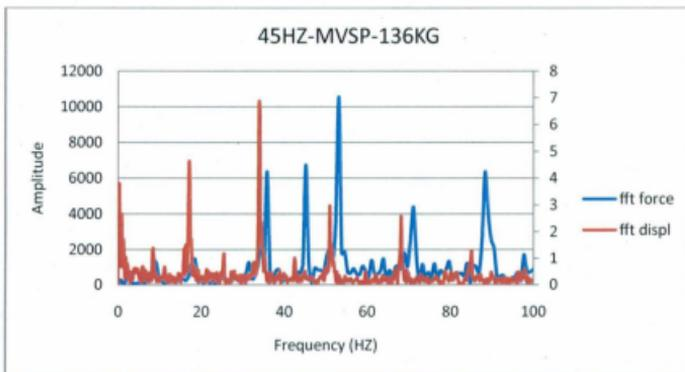
Figure 78. Force and Displacement FFT at 45Hz-MVSP-136Kg
