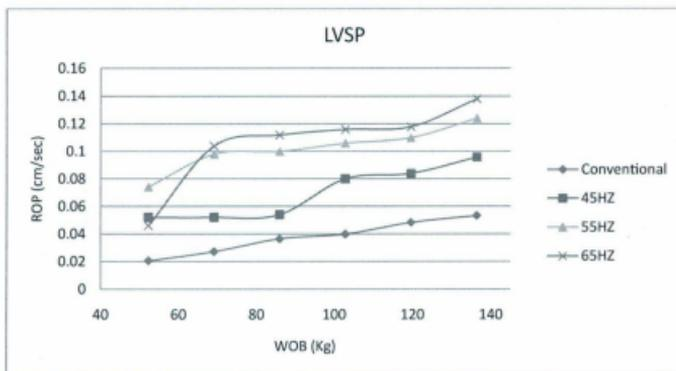
Figure 44. PDC Bit Drilling at LVSP
