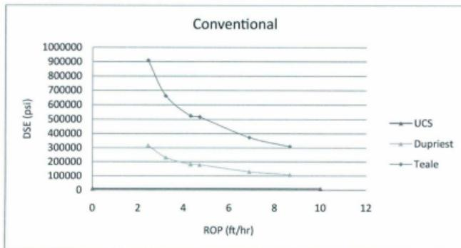
Figure 84. DSE v. ROP for PDC Conventional Drilling
