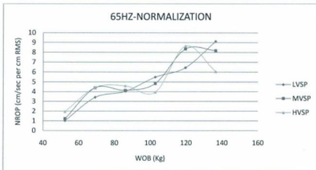
Figure 64. NROP v. WOB at 65Hz Frequency
