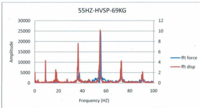
Figure 79. Force and Displacement FFT at 55Hz-MVSP-69Kg
