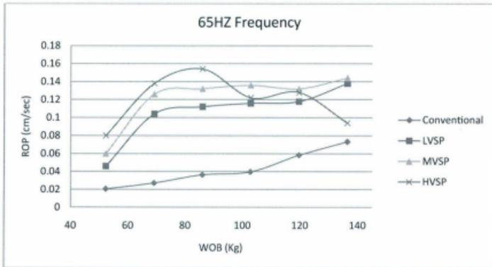
Figure 43. 65HZ PDC Bit Drilling
