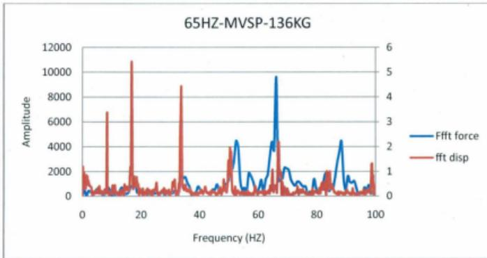
Figure 82. Force and Displacement FFT at 65Hz-MVSP-136Kg
