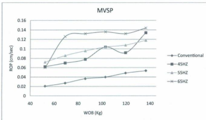
Figure 45. PDC Bit Drilling at MVSP
