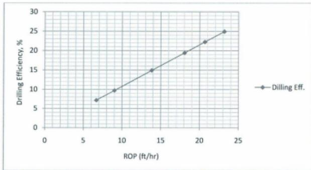
Figure 34. Drilling Efficiency for Conventional Drilling
