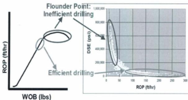
Figure 4. Relationship between the traditional ROP v. WOB plot and the DSE v. ROP plot [13]
