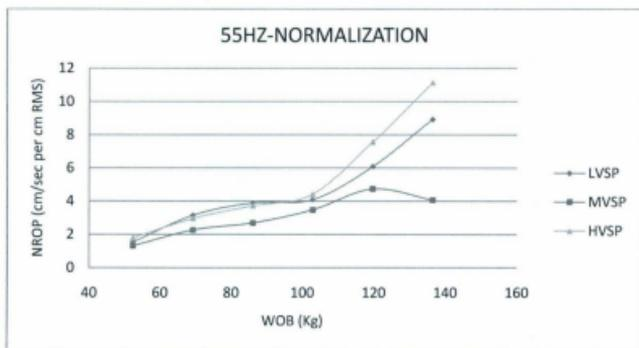
Figure 63. NROP v. WOB at 55HZ Frequency
