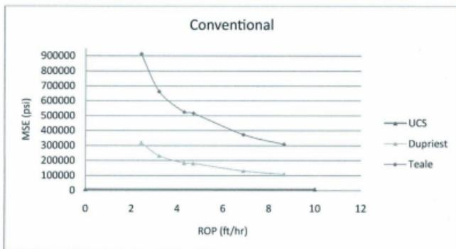
Figure 83. MSE v. ROP for PDC Conventional Drilling
