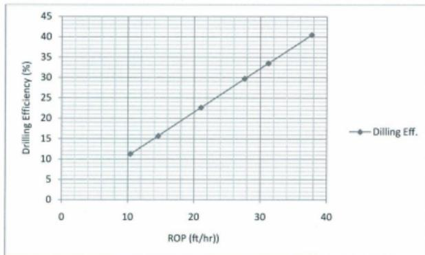
Figure 35. Drilling Efficiency for 55HZ - LVSP Drilling
