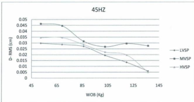
Figure 47. D-RMS v. WOB at 45HZ Frequency
