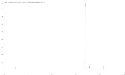
Figure 3.5: HPLC chromatogram of delphinidin-3-glucoside standard
