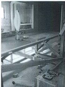
Figure 6.4 Turbine Coupled with Generator in the Wind Tunnel
