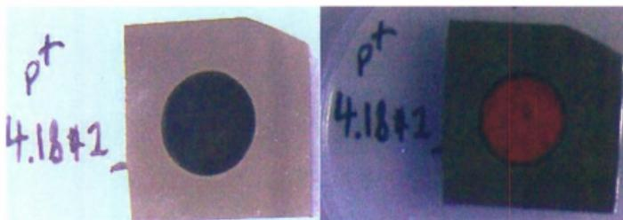
Figure 4-1: Stain etched sample viewed under ultraviolet light.
