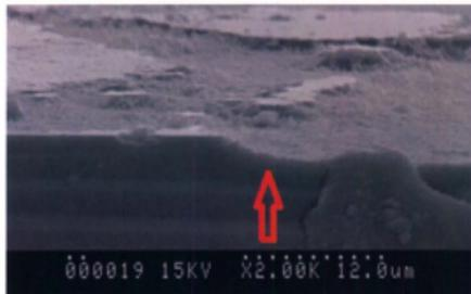
Figure 4-3: SEM of stain etched sample with curvature.
