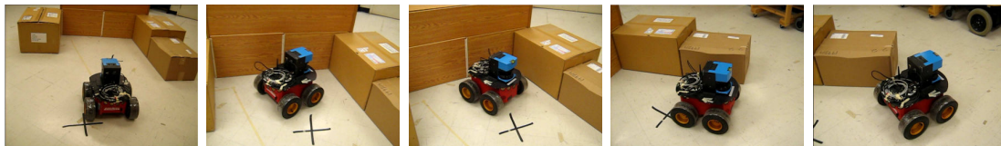
(a) Approaching a subgoal (b) Turning at the dead end (c) Completing the turn (d) Following the wall (e) Turning at the dead end
