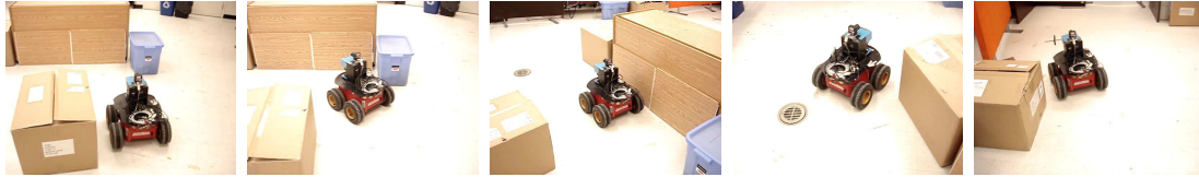
(a) Approaching a subgoal (b) Avoiding the obstacle at front (c) Following the wall (d) Turning at the obstacle (e) Reaching the goal
