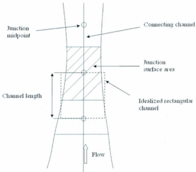
Figure 4.1 Representation of DYNHYD5 model network
