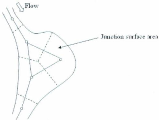
Figure 4 2 Definition sketch for junction surface area
