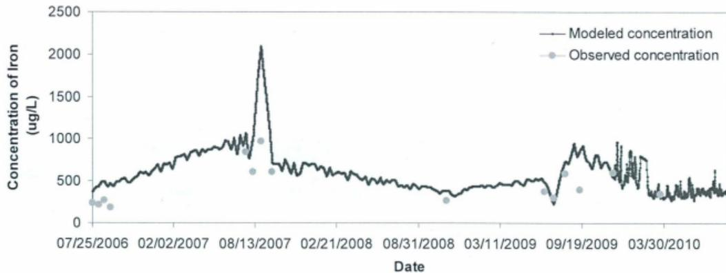
Figure 6 16 Modeled and observed concentrations of Iron for the entire simulation time period (Segment 7)
