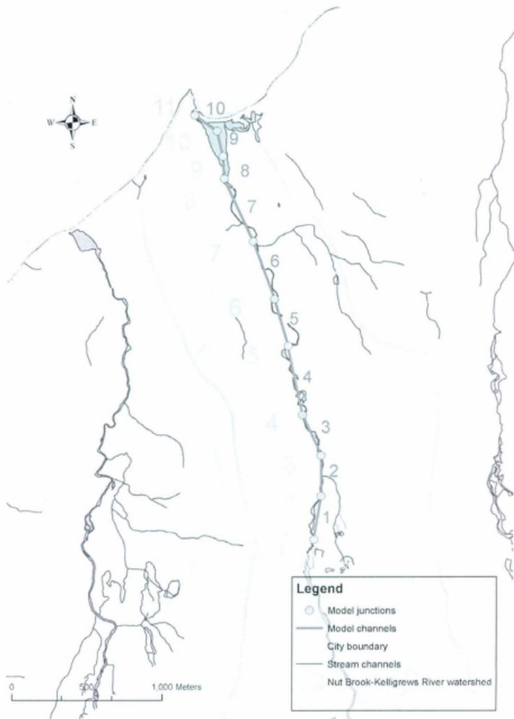
**Figure 5 3 The DYNHYD5 Model network**
