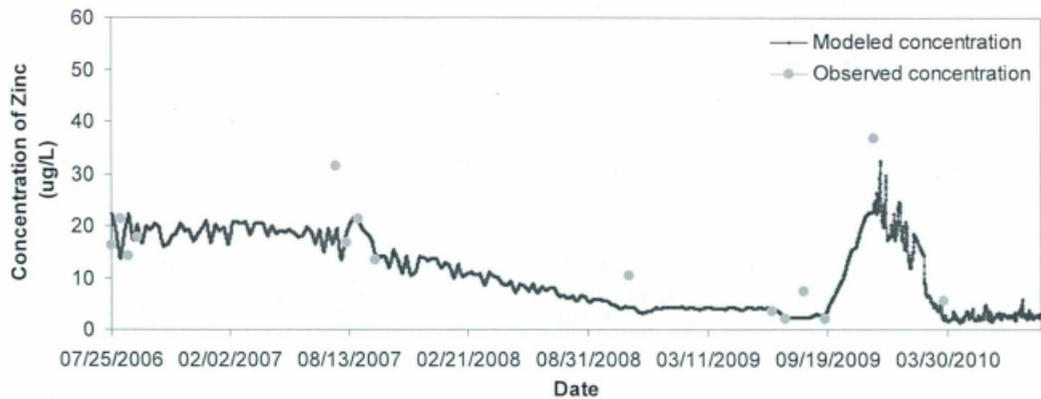
Figure 6 15 Modeled and observed concentrations of Zinc for the entire simulation time period (Segment 7)
