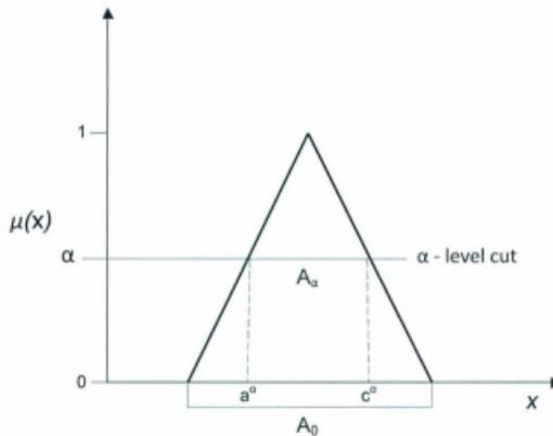
**FIGURE 3.4 - TRIANGULAR FUZZY NUMBER WITH SUPPORT  $A_0$  AND  $\alpha$ -CUT**
