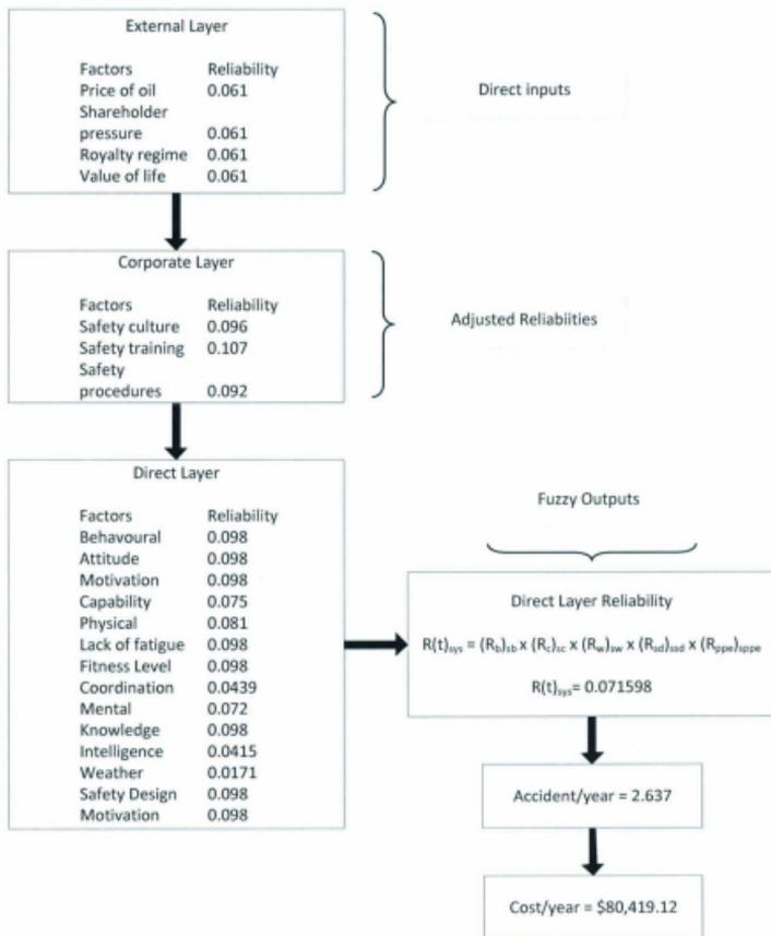
FIGURE 5.4 - PREDICTIVE RUN DISPLAYING MINIMUM FUZZY MODEL OUTPUTS
