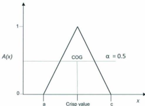
**FIGURE 5.6 - TRIANGULAR MEMBERSHIP FUNCTION REPRESENTING PREDICTED ACCIDENT RATE**
