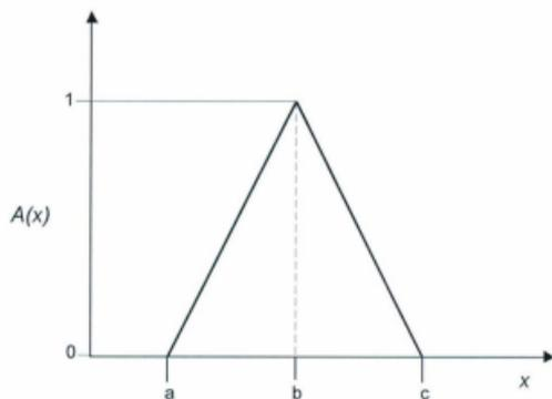
**FIGURE 3.2 - GENERIC, SYMMETRIC, AND TRIANGULAR MEMBERSHIP FUNCTION**
