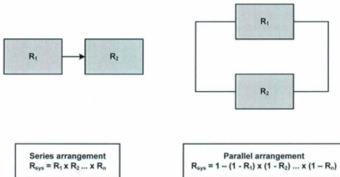
**FIGURE 2.3 - SERIES VERSUS PARALLEL SUBSETS (ATTWOOD ET AL., 2006A)**
