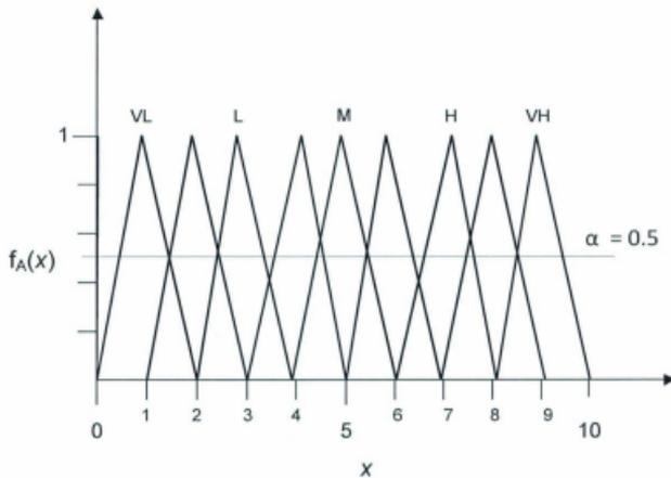
FIGURE 4.2 - TRIANGULAR FUZZY NUMBERS WITH A- CONFIDENCE LEVEL OF 0.5
