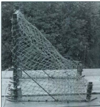
**Figure A.1:** Side view of one of the kelp collection devices that were provided to each fish harvester to collect kelp blades from their fishing boats.
