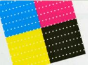
Photogravure is one of the first multiple-producing photographic processes. A photographic image is etched into a copper plate and then printed on an intaglio press. Four-colour photogravure uses four plates, cyan, magenta, yellow and key-line black. When they are printed together, a full colour image is achieved.
