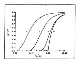
Fig. 3.<sup>26</sup> The dependence of the reduced transition temperature  $T_c(a,b)/T_{c1}$  on the thickness  $a/a_c$ . (a)  $b/a_c = 0.01$ , (b)  $b/a_c = 0.1$ , (c)  $b/a_c = 1.0$  (d) infinite b.
