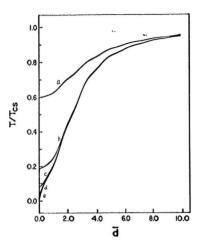
Fig. 7. The dependence of the reduced transition temperature  $T_c/T_c s$  on the thickness  $\bar{d}:=d_s/\xi_0$  for  $T_{cN}=0$  and  $D=\ln(2)/\ln(3)$  with order of the fractal M. (a) M=1, (b) M=2, (c) M=3, (d) M=4, and (e) M=5.
