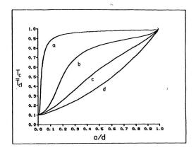
Fig. 4.<sup>26</sup> The dependence of the reduced transition temperature  $T_c(a,b)/T_{c1}$  on the thickness a/d for  $T_{c2}/T_{c1}=0.1$ . (a) $d/a_c=0.05$ , (b) $d/a_c=2.0$ , (c) $d/a_c=7.0$ , and (d)  $d/a_c=50.0$ .
