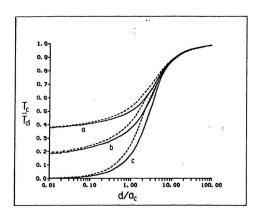
Fig. 5.<sup>26</sup> The dependence of the reduced transition temperature  $T_c(a,b)/T_{c1}$  on the thickness  $d/a_c$  for a=b. (a) $T_{c2}/T_{c1}=0.1$ , (b) $T_{c2}/T_{c1}=0.01$ , and (c) $T_{c3}/T_{c1}=0$ . The corresponding results of the McMillan model are shown by the dotted line.
