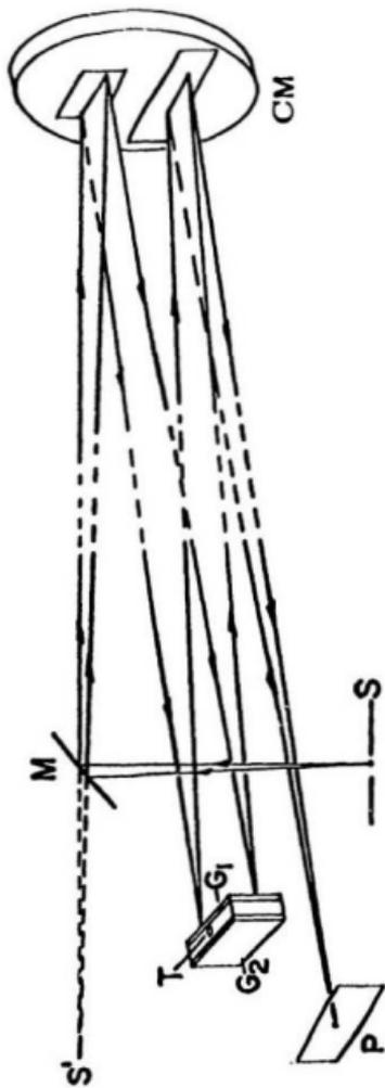
Figure 2.3 Optical layout of the 2 m Bausch and Lomb grating spectrograph with a monochromatic light beam; S': virtual position of S; P: photographic plate; CM: collimating mirror; S: slit; T: rotatable turret; G<sub>1</sub> and G<sub>2</sub>: gratings; M: plane mirror.
