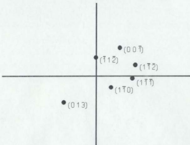
Figure 3.3: Laue diffraction photograph of crystal #3.
