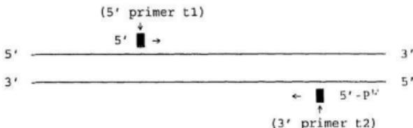
Step 2b. Primer pair is also added for a reference sequence cDNA also present in the same sample. The quantity of this reference sample is always constant. Both the reference and target are co-amplified in the same tube.
