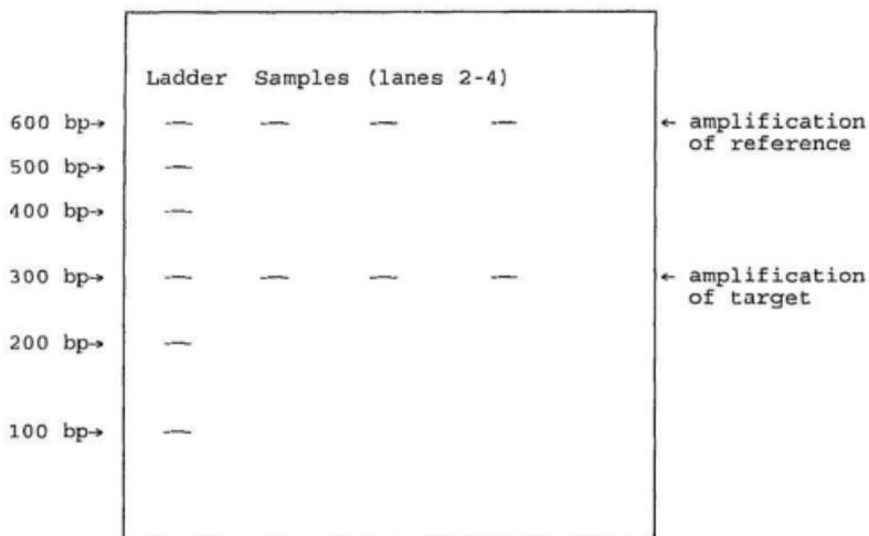
Step 5. The products are excised and counted in scintillation fluid. The counts for the target are normalized to those of the reference.
