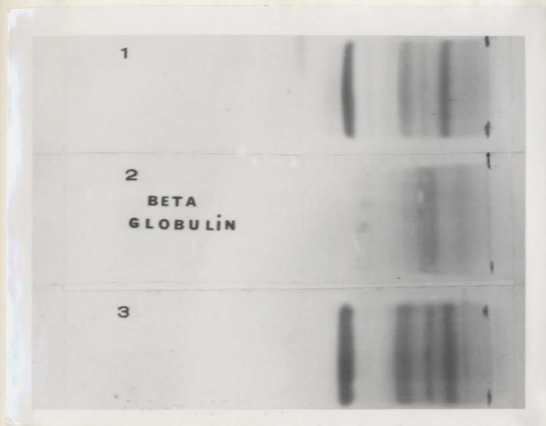
FIGURE 10 CELLULOSE ACETATE ELECTROPHORETIC SEPARATIONS OF PIGLET PLASMA PROTEIN FRACTIONS, WITHOUT AND WITH THE ADDITION OF A PORCINE COHN FRACTION (BETA GLOBULIN)
