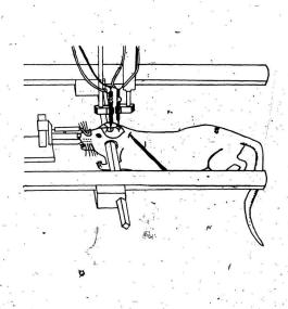
micropipettes were prepared for pressure ejection using the method of Neuman (1986c). PG was ejected (35-137 kPa) using a compressed air source. Other drugs were applied by pressure pulses (50-1000 msec at 275 or 550 kPa) using a Picospritzer connected to a nitrogen gas source.
