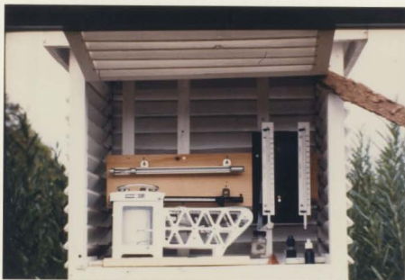
Figure 2-3: Photograph of the contents of the Stevenson screen.
