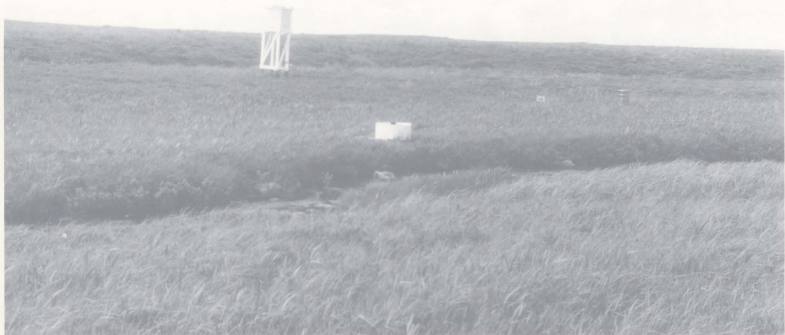
Figure 2.5 Meteorologic Station Showing Location of Stephenson Screen, Precipitation Gauge, and Evaporation Pan. Old Sams River is in the Foreground.
