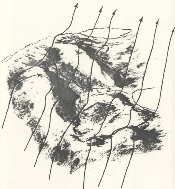
Figure 5.2 Schematic representation of streamlines and vortices, over the Black Mountain area indicated by the deformation of tamarack. View looking northeast.
