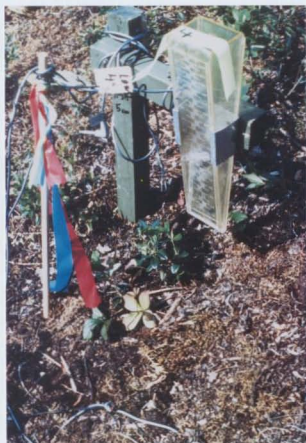
Figure 3-3: Photograph of the fourth pedo-meteorological station, tebuthiuron plot, showing the transparent cumulative wedge-type rain gauge and flag tape marking the apparent depth of the soil moisture and temperature probes.
