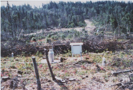
Figure 1-1: Photograph showing the boreal forest in the top of the picture with Gambo Pond in the background. In the foreground of this south-facing view is the meteorological station showing the continuous recording rain gauge, Stevenson Screen and two white, cumulative, cylindrical rain gauges diagonally opposite of each other. The station is just below the top of the ridge. Behind the meteorological station is the picloram plot where, in the lower end, the field assistant is clearing away slash.
