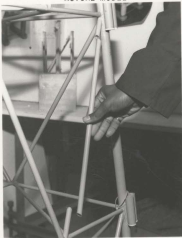
FIG. 5.13 SEVERED MEMBER(S) IN THE ACTUAL AND SIMULATED MODEL.
