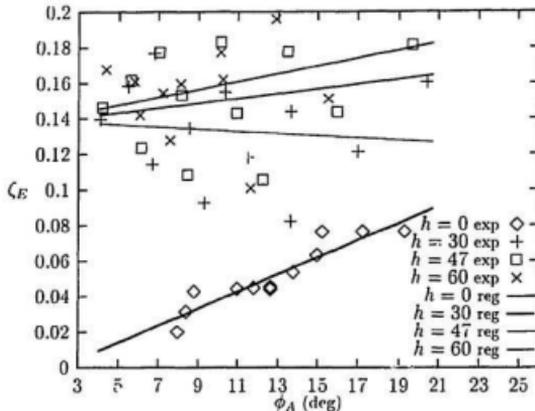
Figure 3.5:  $\zeta_E$  of M36G, tank with damping,  $\omega_\phi = 3.00$
