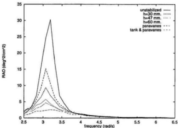
Figure 5.11: RAOs for damped tank,  $\omega_\phi = 3.00$ ,  $(h_w)_{1/3} = 9.8$
