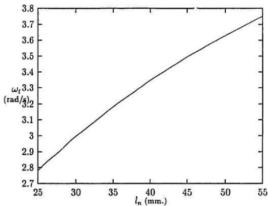
Figure 2.3:  $\omega_t$  vs.  $l_n$ ,  $l_t = 85$ ,  $b_n = 220$ ,  $h = 50$
