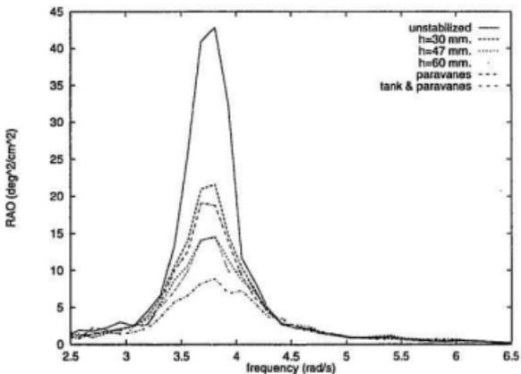
Figure 5.7: RAOs for damped tank,  $\omega_\phi = 3.75$ ,  $(h_w)_{1/3} = 9.5$
