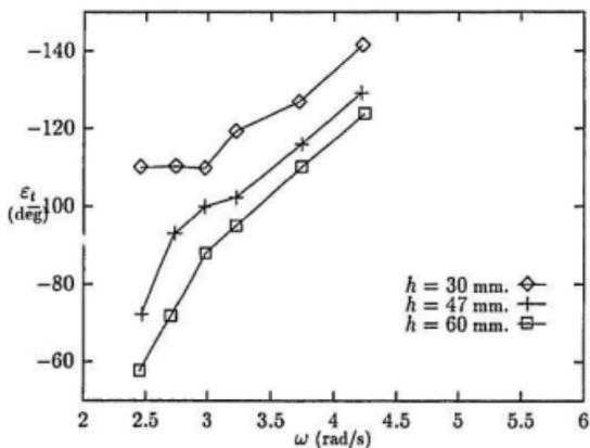
Figure 4.8: Phase lags of damped tank,  $\omega_\phi = 3.00$ ,  $h_w = 5$
