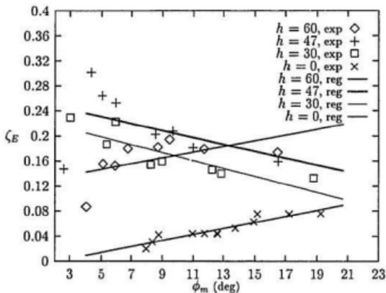
Figure 3.7:  $\zeta_E$  of M366, tank without damping,  $\omega_\phi = 3.00$
