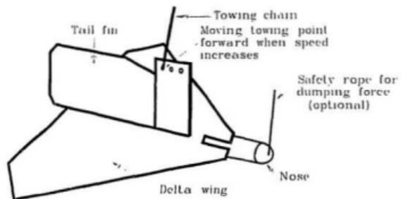
Figure 1.2: The shape of a paravane
