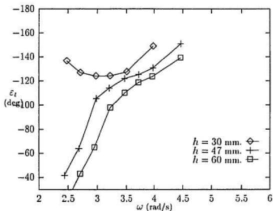
Figure 4.18: Phase lags of undamped tank,  $\omega_\phi = 3.00$ ,  $h_w = 5$
