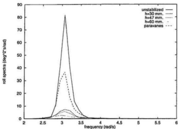
Figure 5.12: Roll spectra for damped tank,  $\omega_\phi = 3.00$ ,  $(h_w)_{1/3} = 4.7$
