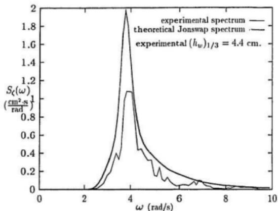
Figure 5.2: Wave spectra for  $\omega_0 = 3.75$  and  $(h_w)_{1/3} = 5$
