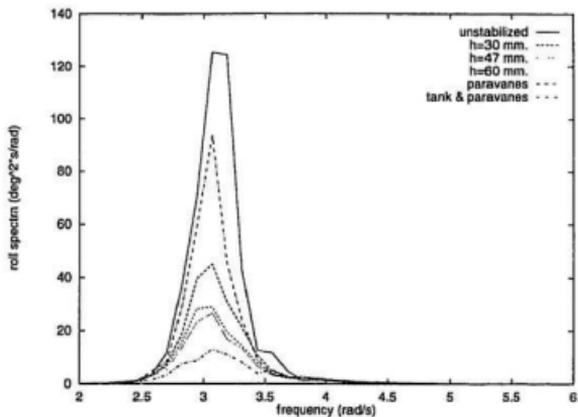
Figure 5.10: Roll spectra for damped tank,  $\omega_\phi = 3.00$ ,  $(h_w)_{1/3} = 9.8$
