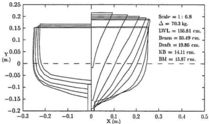
Figure 3.1: Body plan and particulars of Model 366
