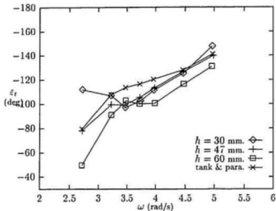
Figure 4.15: Phase lags of undamped tank,  $\omega_\phi = 3.75$ ,  $h_w = 10$
