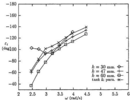
Figure 4.17: Phase lags of undamped tank,  $\omega_\phi = 3.00$ ,  $h_w = 10$
