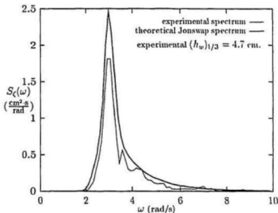
Figure 5.4: Wave spectra for  $\omega_0 = 3.00$  and  $(h_w)_{1/3} = 5$
