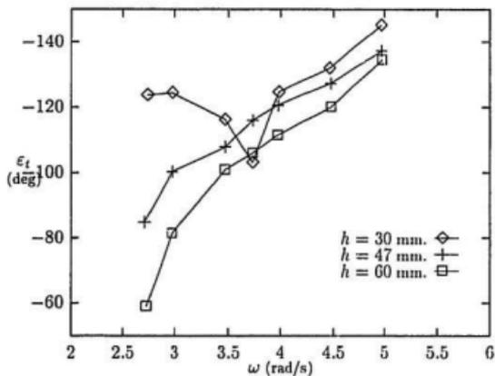
Figure 4.6: Phase lags of damped tank,  $\omega_\phi = 3.75$ ,  $h_w = 5$
