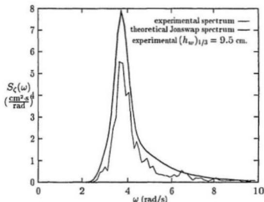
Figure 5.1: Wave spectra for  $\omega_0 = 3.75$  and  $(h_w)_{1/3} = 10$
