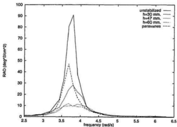
Figure 5.9: RAOs for damped tank,  $\omega_\phi = 3.75$ ,  $(h_w)_{1/3} = 4.4$
