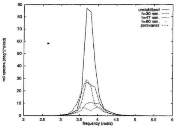
Figure 5.8: Roll spectra for damped tank,  $\omega_\phi = 3.75$ ,  $(h_w)_{1/3} = 4.4$
