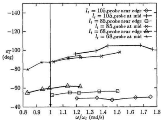
Figure 2.15: Comparison of different probe positions with high damping
