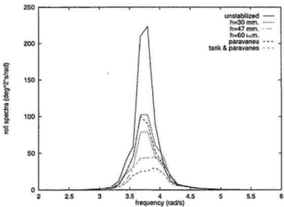
Figure 5.6: Roll spectra for damped tank,  $\omega_\phi = 3.75$ ,  $(h_w)_{1/3} = 9.5$
