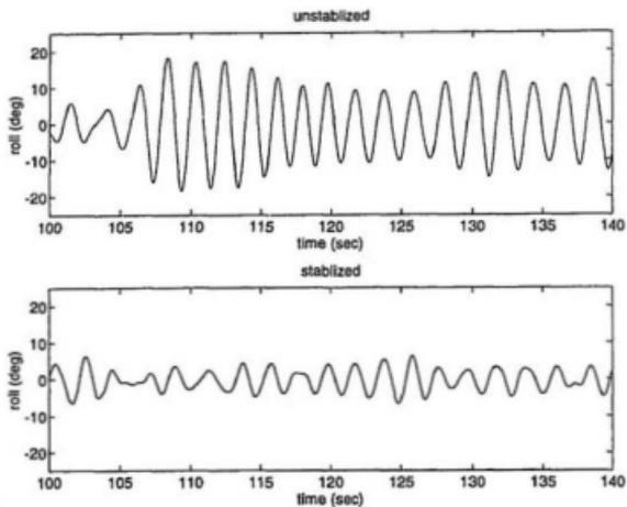
Figure 5.5: Roll samples for irregular wave tests
