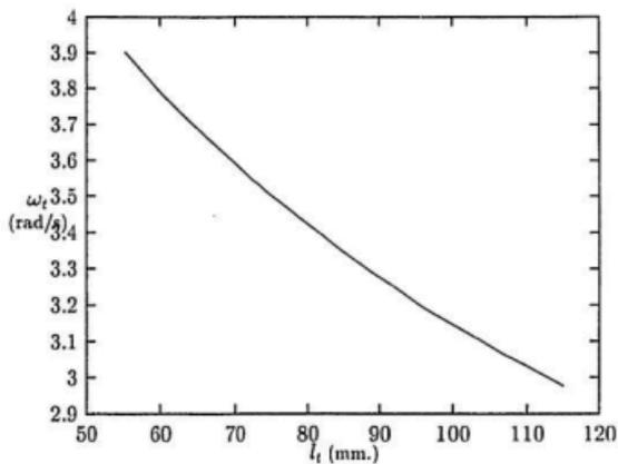
Figure 2.2:  $\omega_t$  vs.  $l_t$ ,  $l_n = 40$ ,  $b_n = 220$ ,  $h = 50$
