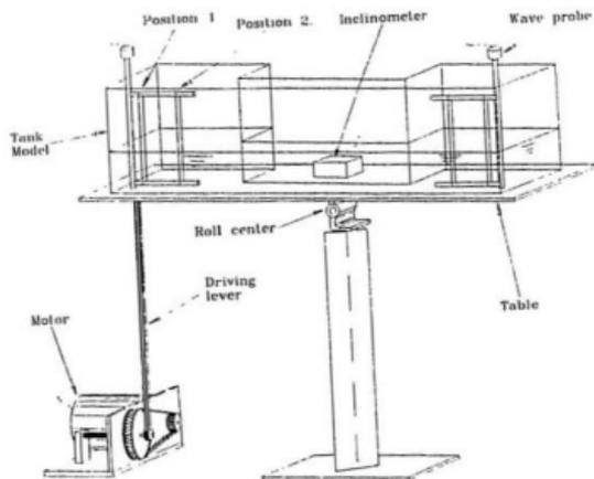
Figure 2.7: Oscillating bench test setup
