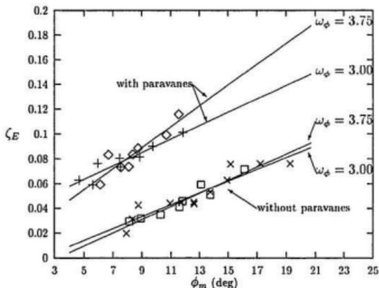
Figure 3.8:  $\zeta_E$  of M366 with paravanes
