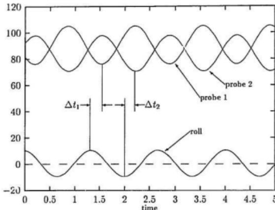
Figure 2.10: Fits of tank-water elevations and roll motions
