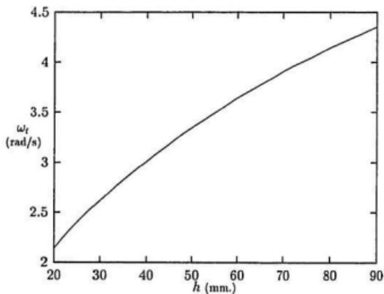
Figure 2.5:  $\omega_t$  vs.  $h$ ,  $l_t = 85$ ,  $l_n = 40$ ,  $b_n = 220$
