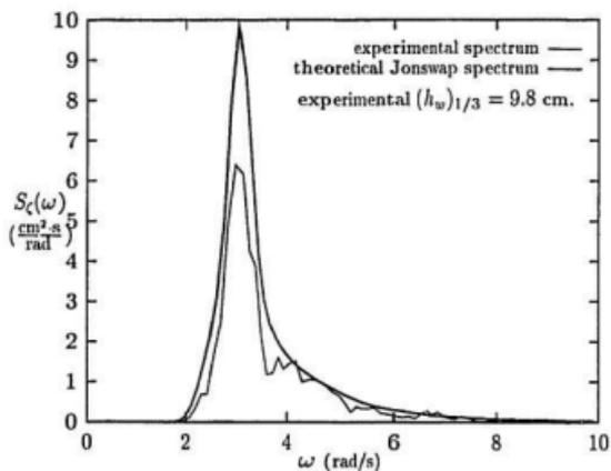
Figure 5.3: Wave spectra for  $\omega_0 = 3.00$  and  $(h_w)_{1/3} = 10$
