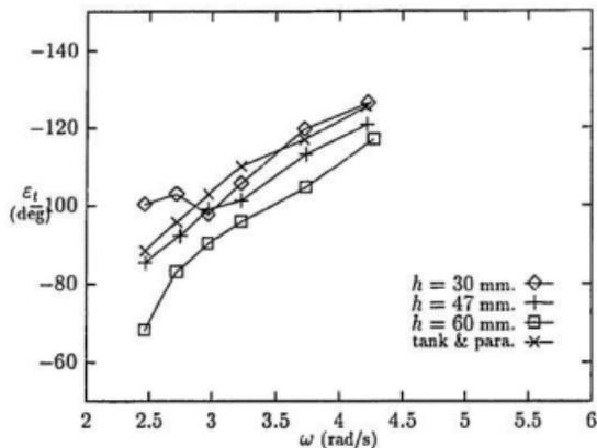
Figure 4.7: Phase lags of damped tank,  $\omega_\phi = 3.00$ ,  $h_w = 10$
