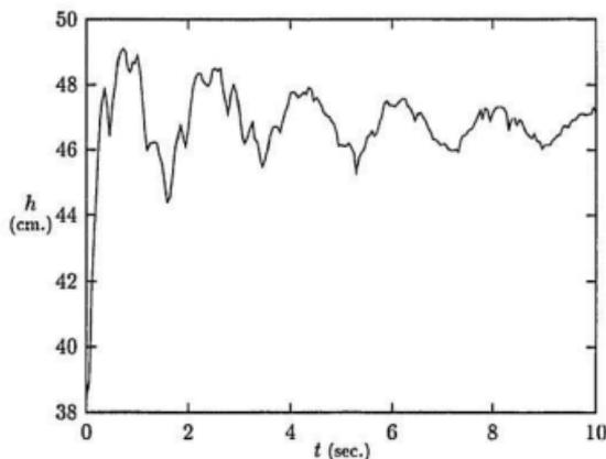
Figure 2.8: A tank decay test for obtaining natural frequency
