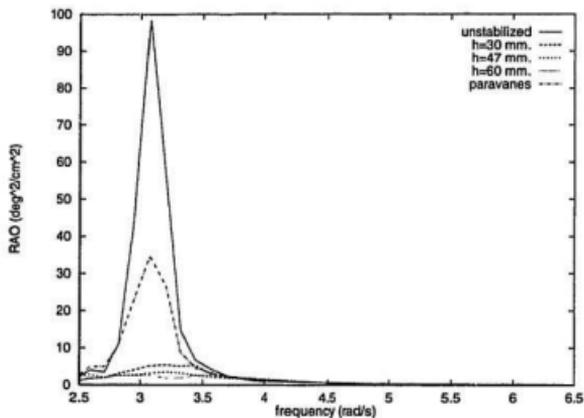
Figure 5.13: RAOs for damped tank,  $\omega_\phi = 3.00$ ,  $(h_w)_{1/3} = 4.7$
