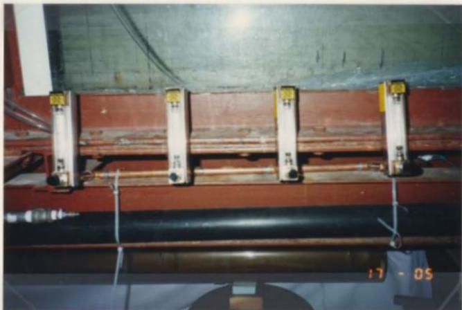
Figure 3.4. Photograph of the flowmeters model # 10A6731N
