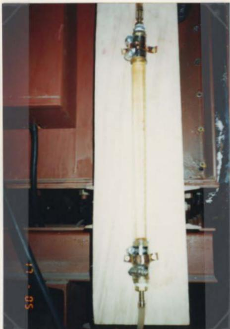
Figure 3.5. Photograph of the flowmeter model # FP-1/2-21-G-10/77
