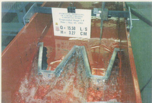
Figure 5-15 Photograph shows the location of depth measuring section
