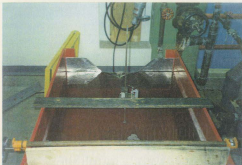
Figure 5-18 Flow depth measurement at the V-notch weir in progress
