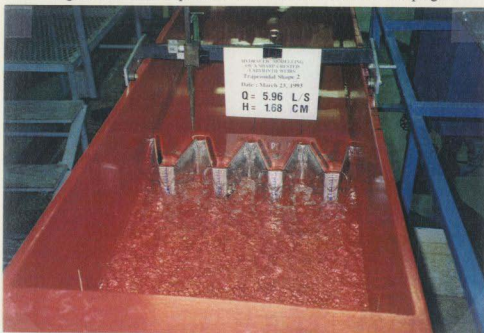
Figure 5-19 Depth measurement at the weir model in progress
