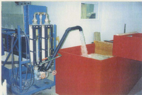
Figure 5-25 Calibration of the V-notch weir in progress
