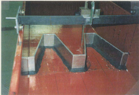
Figure 5-14 Photograph of a thin layer of duxseal along the bottom and sides
