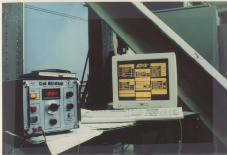
Figure 3.5: The Crack Micro Gauge and MDT testing software screen.
