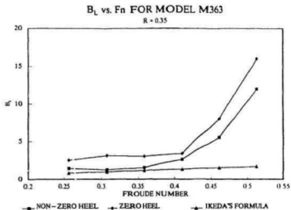
Figure 21  $B_L$  vs.  $F_n$  for M363 with R=0.35
