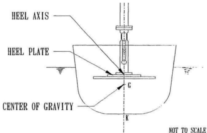
**Figure 5** Positions of heel axis and center of gravity
