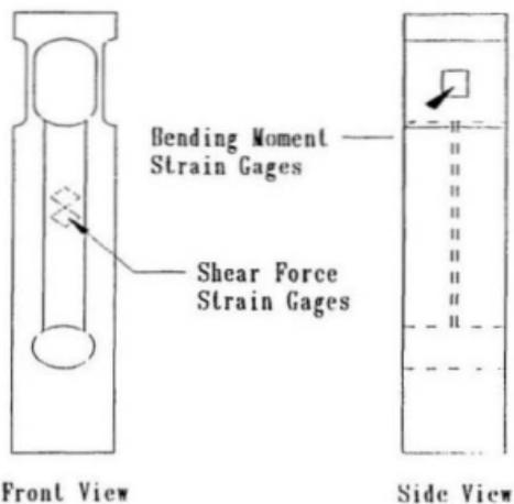
**Figure 1** Measuring element
