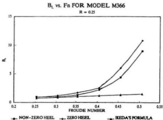
Figure 24  $B_L$  vs.  $F_n$  for M366 with R=0.25
