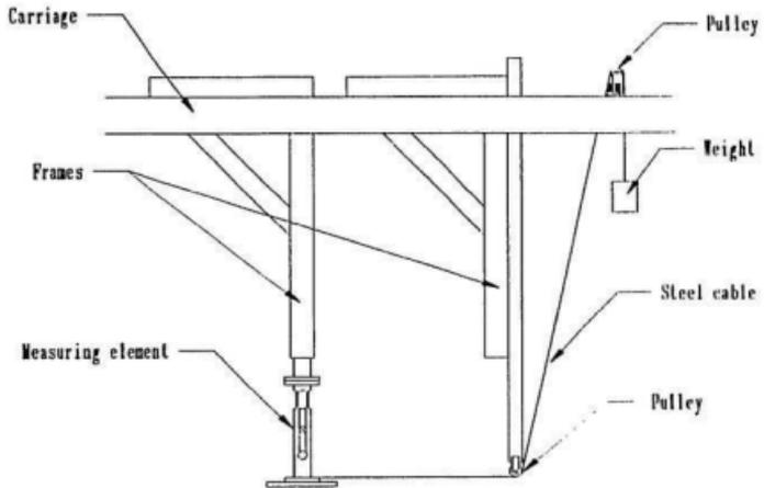
**Figure 6 Calibration setup**
