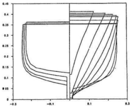
**Figure 4** Lines plan of ship model M366
