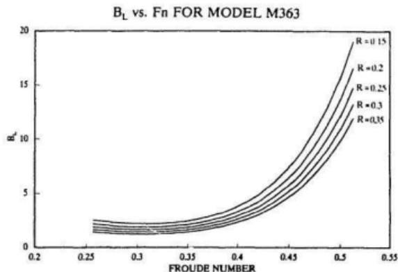
Figure 20(a)  $B_L$  vs.  $F_n$  for M363 at different  $R$  values
