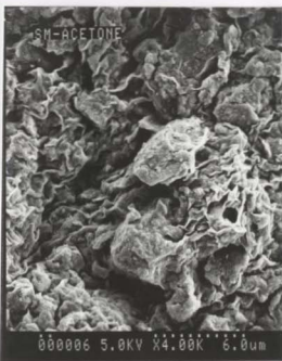
Figure 4.13: Photomicrographs of Smectite – (a) Water (b) Acetic acid (c) Aniline (d) Acetone
