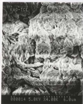
Figure 4.10: Photomicrographs of Kaolinite – (e) Methanol (f) CTC (g) TCE (h) Xylene
