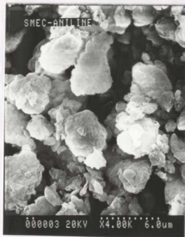
Figure 4.13: Photomicrographs of Smectite – (a) Water (b) Acetic acid (c) Aniline (d) Acetone
