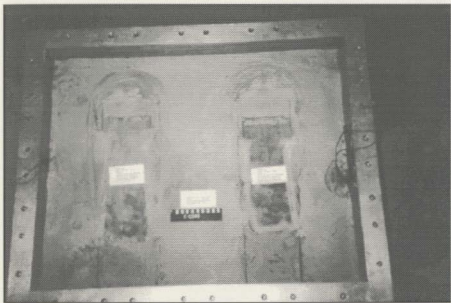
Figure 7.1 Plan View of Model Testbed Showing Scours C (Left) and D (Right)
