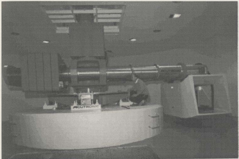
Figure 5.1 The 680-2 Acutronic Geotechnical Centrifuge At Rest
