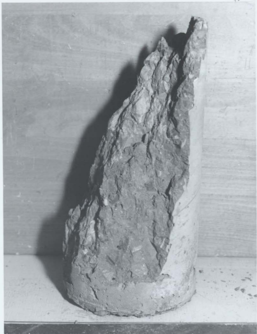
Figure 3.2: Failure surface of a high-strength concrete cylinder
