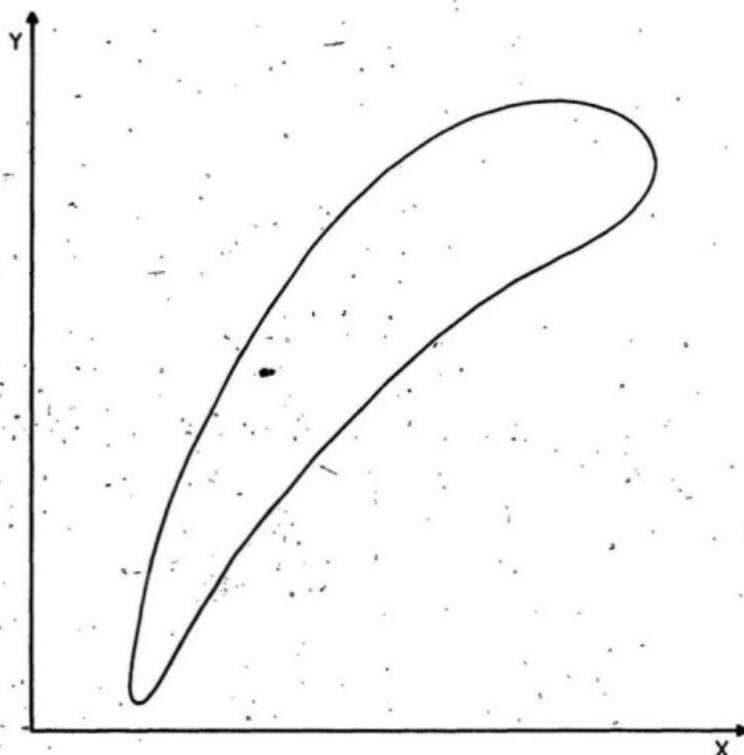
Fig. C.3 The Turbine Blade Airfoil Cross-section at  $Z=0.05\text{ m}$ .
