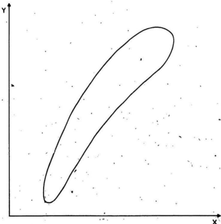
Fig. C.4 The Turbine Blade Airfoil Cross-section at  $Z=0.075\text{ m}$
