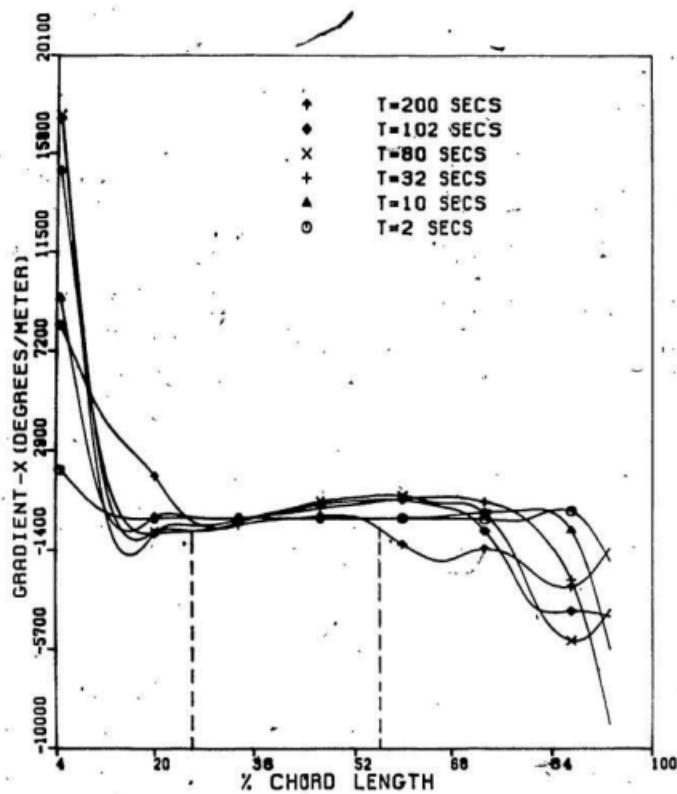
FIG. 2.7 THE VARIATION OF THE TEMPERATURE GRADIENT-X ALONG THE MID-SECTION (2-2') AT  $T_g = 870^\circ\text{C}$ .
