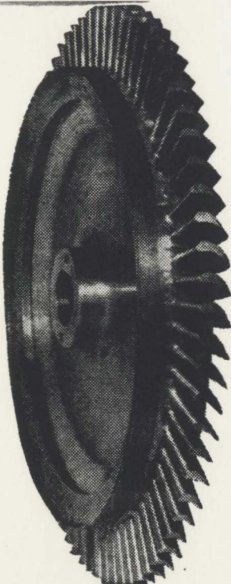
FIG.1.2a THE GAS TURBINE DISK-BLADE ASSEMBLY [2]
