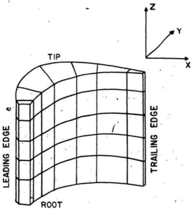
FIG.3.3 The turbine blade finite element model
