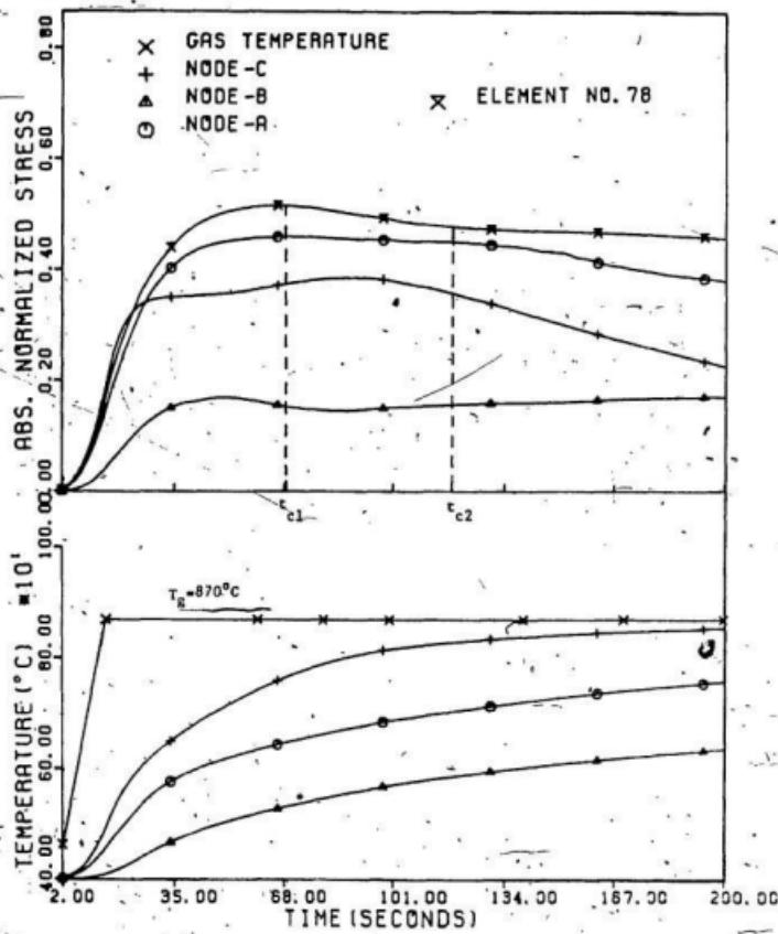
FIG.4.2 THE TRANSIENT TEMPERATURE AND THERMAL STRESS DISTRIBUTION IN THE BLADE FOR THE FEASIBLE HEATING RATE OF 31.33 C/SEC & FINAL  $T_g = 870^\circ\text{C}$
